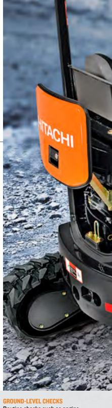
Routine checks such as engine oil level are quickly accomplished from ground level. Convenient lube/maintenance chart helps ensure that nothing gets overlooked.
