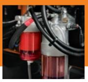
■ Engine oil, fuel and hydraulic pilot oil filters are all located on the same side at ground level for easy servicing.
