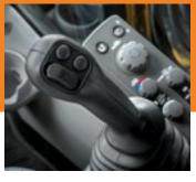
■ Ergonomically correct shortthrow pilot levers provide smooth, precise control with less effort. Pushbuttons in the right lever allow control of auxiliary hydraulic flow for attachments. Optional sliding switch provides proportional speed control, giving you full command from your fingertips.
