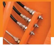
Centralized lube banks place zerks within easy reach, making greasing less messy and timeconsuming.
