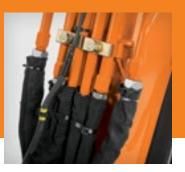
■ Steel hydraulic lines are clamped securely, and wear-resistant hoses are protected with Cordura® covering.
