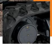
■ Unique steel cores within rubber tracks resist cracking, and large-diameter drive sprockets and track idlers make for a rock-solid undercarriage.
