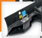
■ Redesigned blade extension pins allow you to effortlessly expand the width of the blade to match the track width on the ZXI7U-5.
