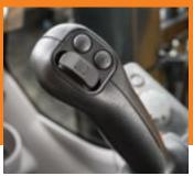
Ergonomically correct short-throw pilot levers provide smooth, precise fingertip control with less movement or effort. Standard sliding switch provides proportional speed control, giving you full command from your fingertips.
