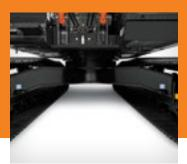
■ Box-section track frames, thickplate single-sheet mainframe, and superior ground clearance and industry-exclusive double-seal swing bearing deliver rock-solid durability.
