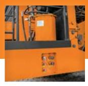
■ Hitachi trucks feature a fastfill system station. This station,
