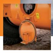
■ The collapsible step and flat service stage inside the rear axle brings higher serviceability and safety.
