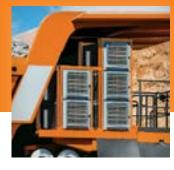
■ The AC-drive system has multiple controls that ensure trouble-free reliability and less maintenance. They include grid dry motor control that keeps the grid system dry in cold or wet conditions. A blower control cools the alternator and wheel motors in hot conditions.
