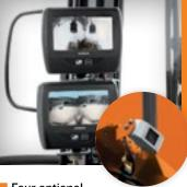
Four optional outside cameras can be mounted around the machine for enhanced visibility and help eliminate blind spots.
