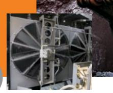
Two oil coolers are strategically positioned far from the engine radiator for even better cooling potential.
