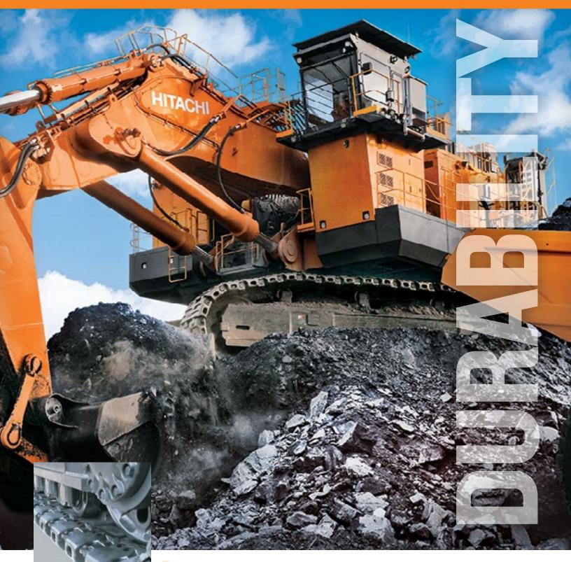
Rugged track links include roller guides to help extend service life.
