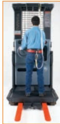
**Wrap-around compartment** provides clear wide view of racks, aisles and pick locations.
