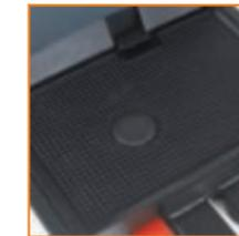
**Low-effort, flush-mounted brake pedal** allows increased freedom of movement for greater operator comfort.
