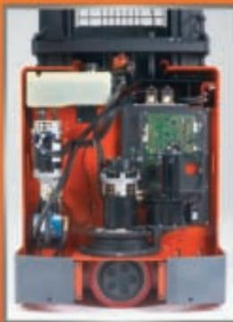
**Power unit tractor cover** is easily removed to provide access to major components, reducing service time during inspection and maintenance.
