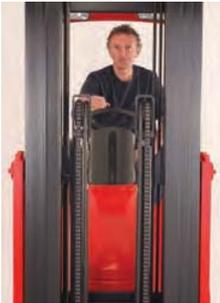
Operators have excellent forward visibility thanks to the triplex free lift mast, with its twin side mounted lift cylinders. Mast tilt means easy fork entry into pallets.
