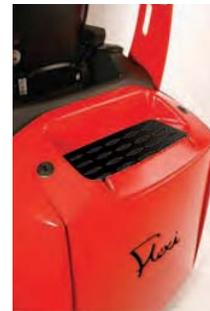
Conveniently located behind the operator and suitable for carrying a roll of plastic film or any other material that needs to be close to hand.
