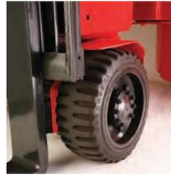
Four large cushion rubber tires deliver optimum performance and traction. They're also resistant to damage which means a long service life and less downtime.
