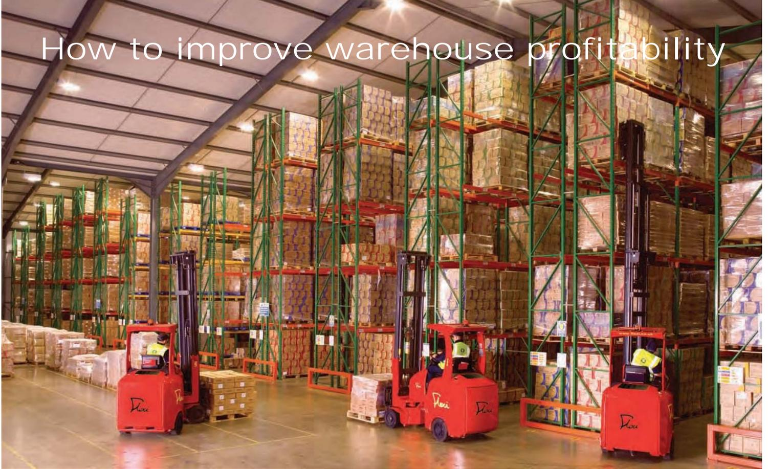
**Flexi** works in just 6 feet aisle widths - liberating a potential **30% more** warehouse capacity compared with conventional reach trucks.
