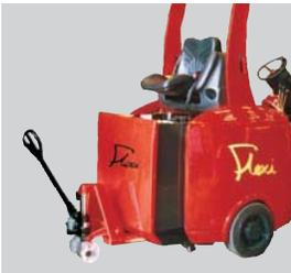
Low rear lift off or roll off for fast changeovers. Good access for battery topping. No motors underneath.
