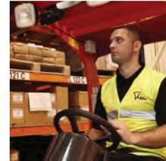
High definition LCD CCTV allows operator to stack safely up to 32 feet with minimum fatigue. Programmable lift height selection for fast stacking.
