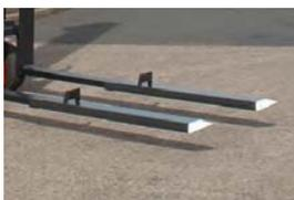
Telescopic double deep fork attachment provides extra 50% storage capacity over reach trucks for true bulk store operations.
